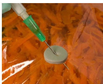
Septum perforated by a hollow needle.
