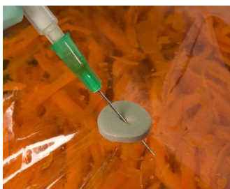
Septum perforated by a hollow needle.
